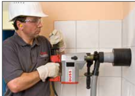
Dry drilling in a chimney pipe with dust extraction, hand-held
